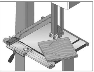
Figure 55. Example of a stacked cut setup.
